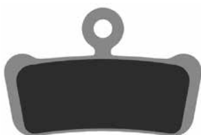
Organic / Sintered DBP-57 / DBP-57S DBP-57E organic + kevlar, for E-bike
